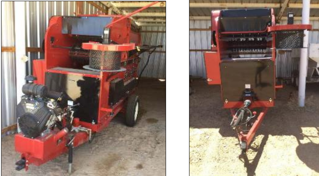
Figure 2. Hopster hops picker manufactured in Pennsylvania. Delivered in June 2017. The Hopster 5G (upper left) is powered by a gasoline generator. The Hopster 5P (upper right) is powered by tractor power take-off (PTO). Both units are mobile. The picker fingers and dribble belts (bottom). NMSU Agricultural Science Center at Farmington, NM. 2017.
